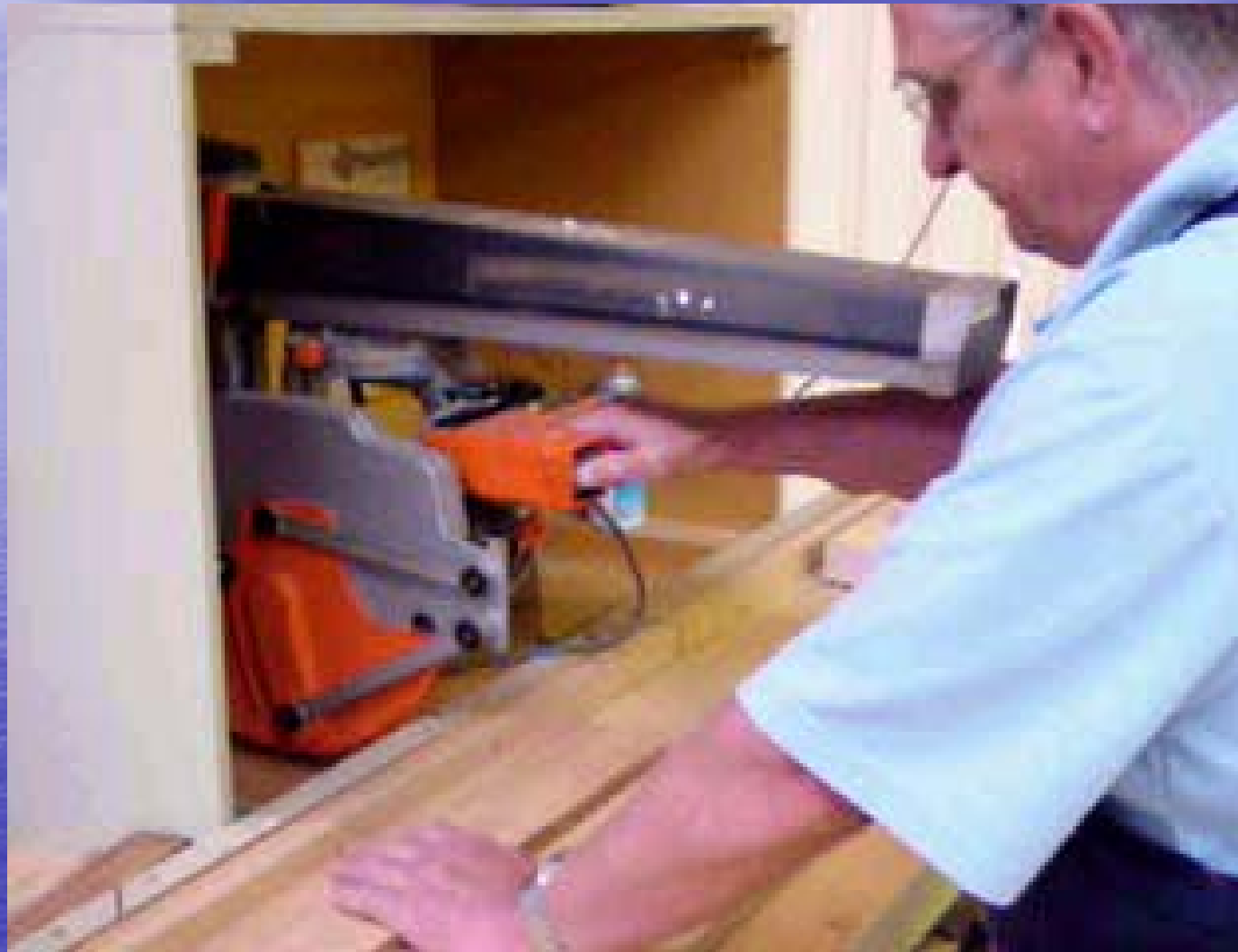
Self Adjusting Guard - Radial Arm Saw
